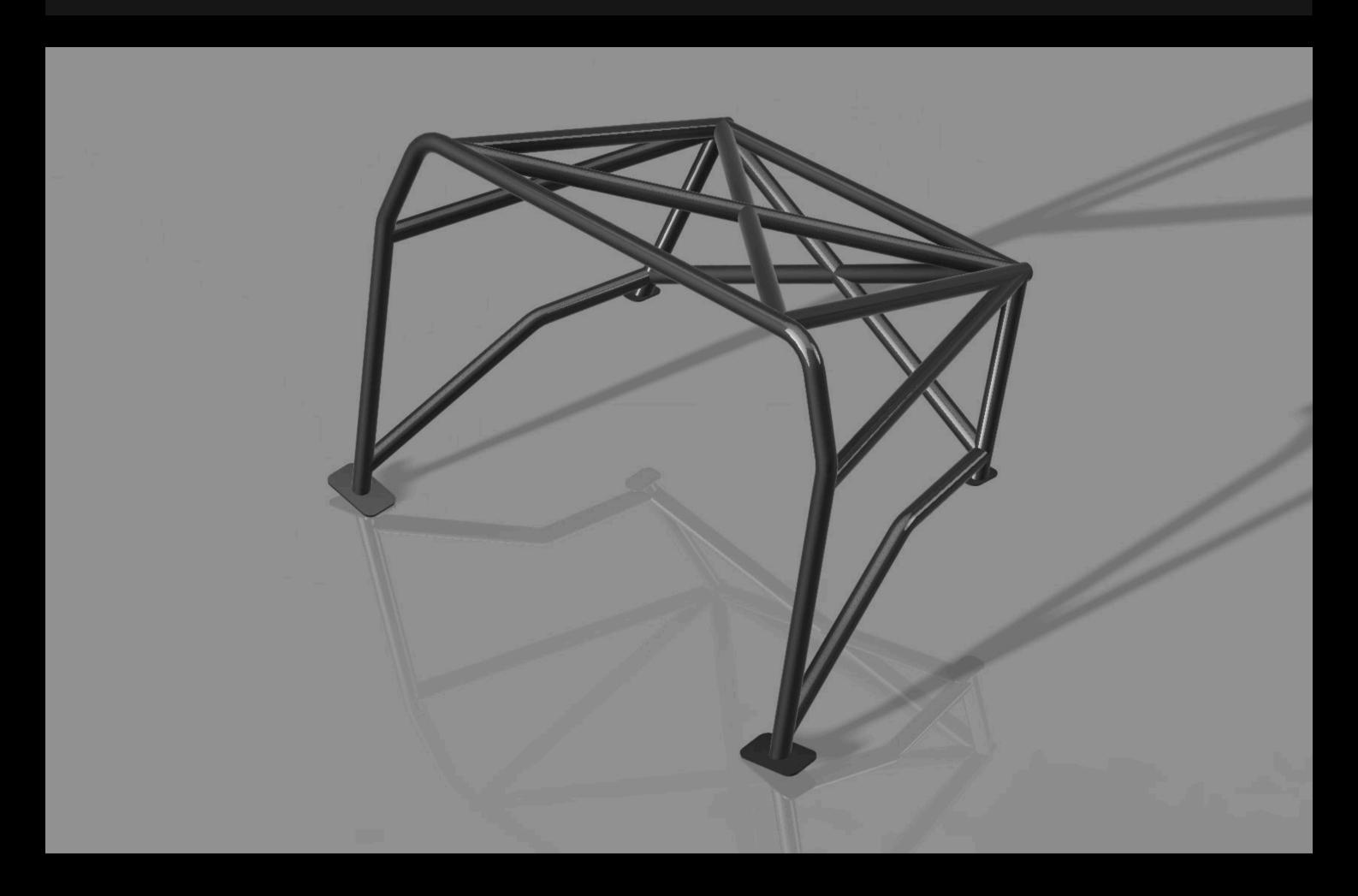
The safety cage for classic Ford Mustangs has been designed to combine the authentic character of the iconic car with modern engineering solutions. The structure was developed based on detailed 3D CAD models and precise laser scans of factory bodies, which allowed for a perfect fit. It is made of S355 steel - a material renowned for its strength and resistance to extreme loads.
