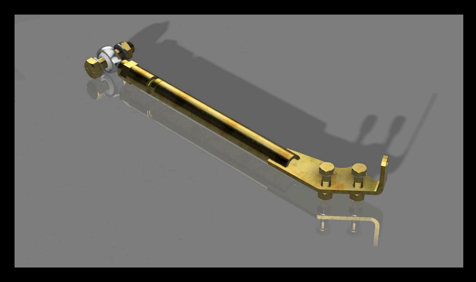
A durable and precise right diagonal control arm specifically designed for classic Ford Mustang models. Its design focuses on combining high stiffness, durability, and adjustability, making it an ideal alternative to the standard suspension. Installation is completely hassle-free—the part fits "plug & play" with no need for any modifications to the bodywork.
