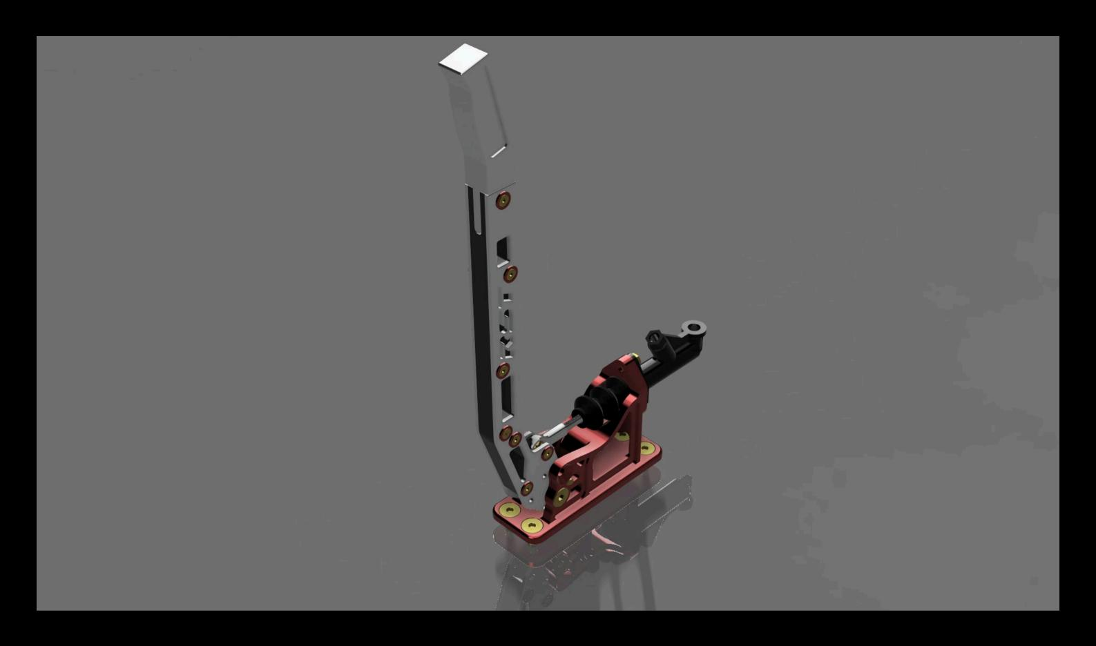
The hydraulic handbrake is an essential tool in any car built for drifting, rallycross, or time attack, where precise rear-end control determines both performance and driving style. Our design was developed with maximum durability, effectiveness, and ergonomics in mind. The project is compatible with the Wilwood GS Compact master cylinder series. Features a removable grip, allowing for various configuration options.
