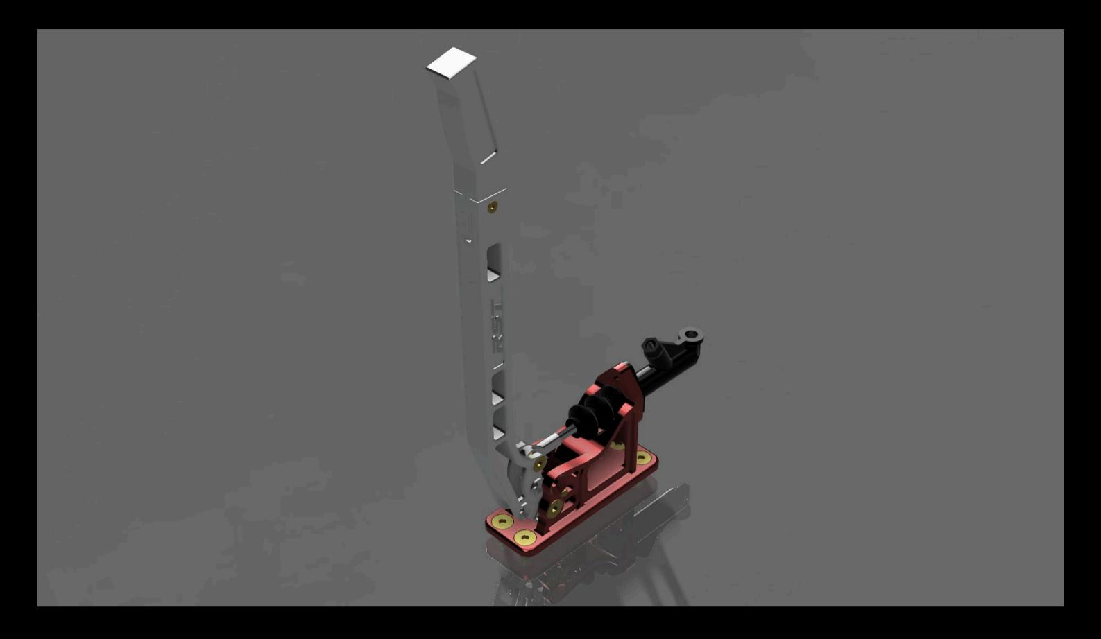
The hydraulic handbrake is an essential tool in any car built for drifting, rallycross, or time attack, where precise rear-end control determines both lap times and driving style. Our design was developed with maximum durability, effectiveness, and ergonomics in mind. The project is compatible with the Wilwood GS Compact master cylinder. Features a removable grip, allowing for various configuration options.
