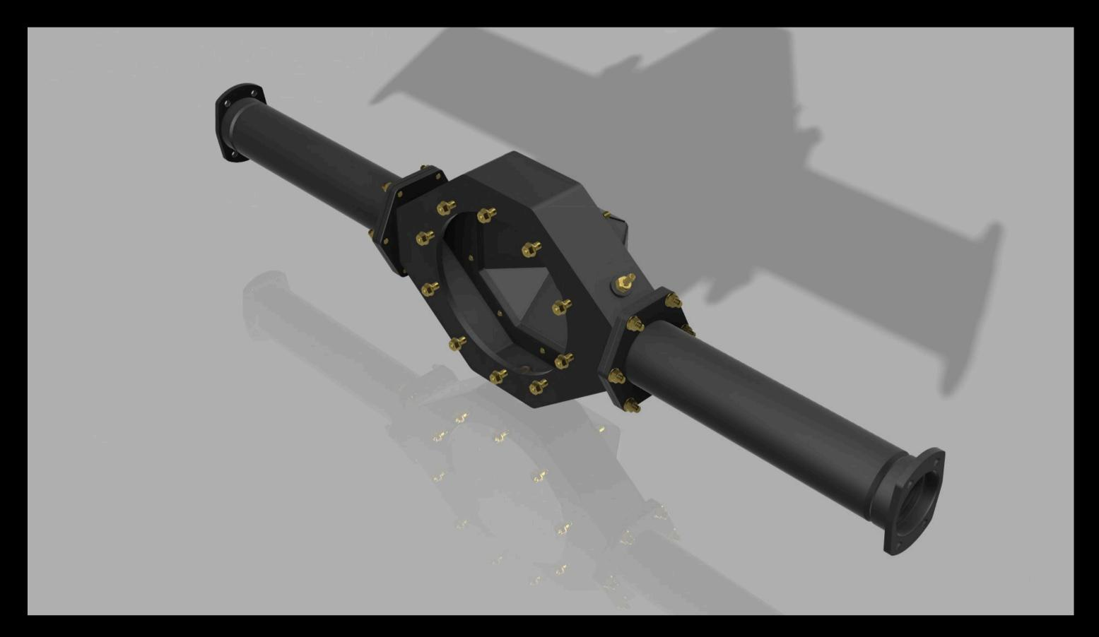
Custom axle housing tailored for the 9-inch C7AWE differential. Engineered for maximum durability, it excels in applications where high torque and strong traction impose particularly demanding requirements on components. The entire system is designed to handle torque up to 1000 Nm. Its modular construction not only simplifies the assembly of the complete set but also allows for various axle width configurations by adjusting the length of the housings.
