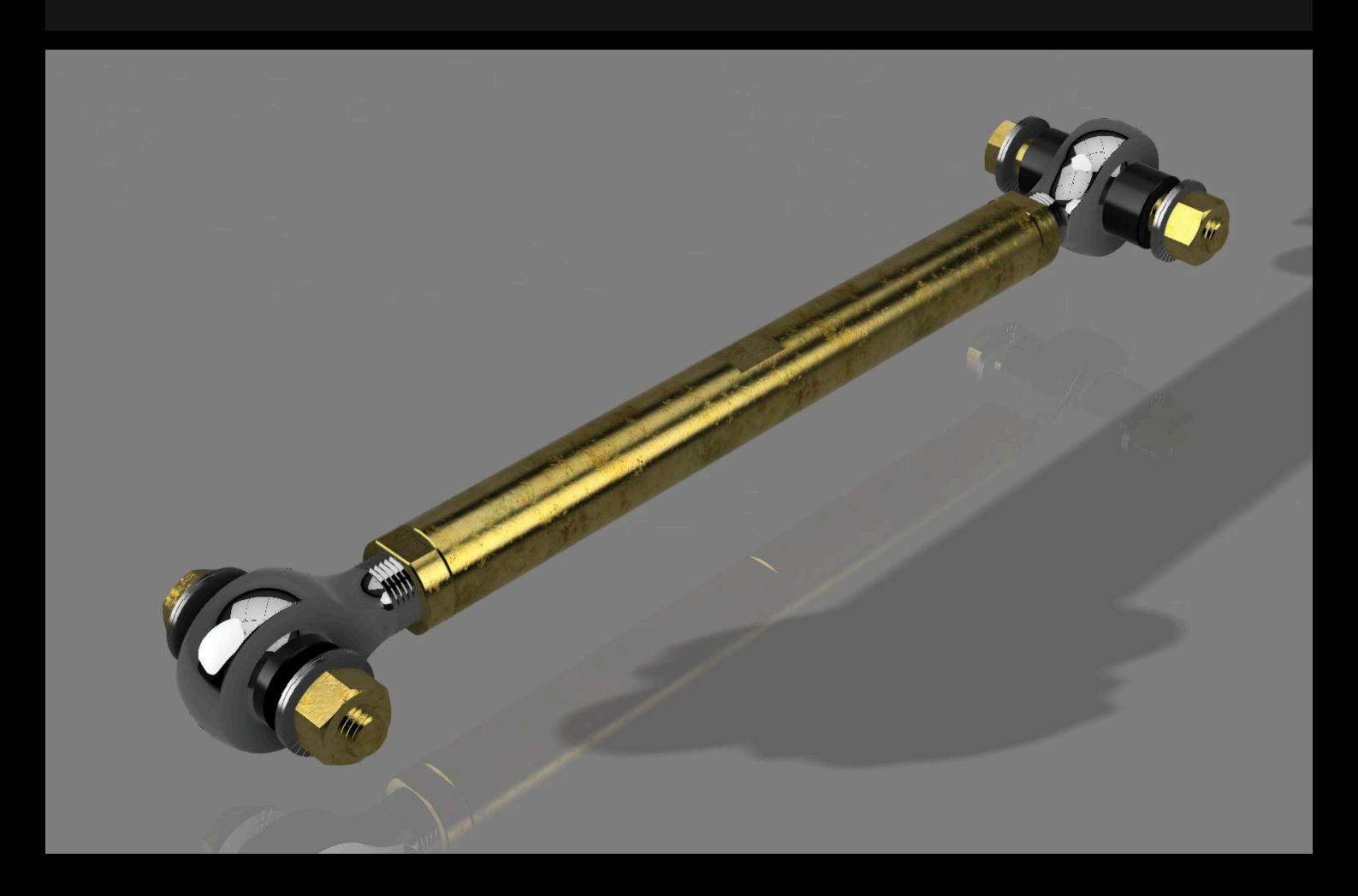
The custom trailing arm has been designed to eliminate common issues often found in factory suspension setups. Its innovative construction is based on the use of uniball spherical bearings, which not only allow for precise adjustment of the arm's overall length but also significantly improve structural rigidity compared to traditional metal-rubber bushings.
