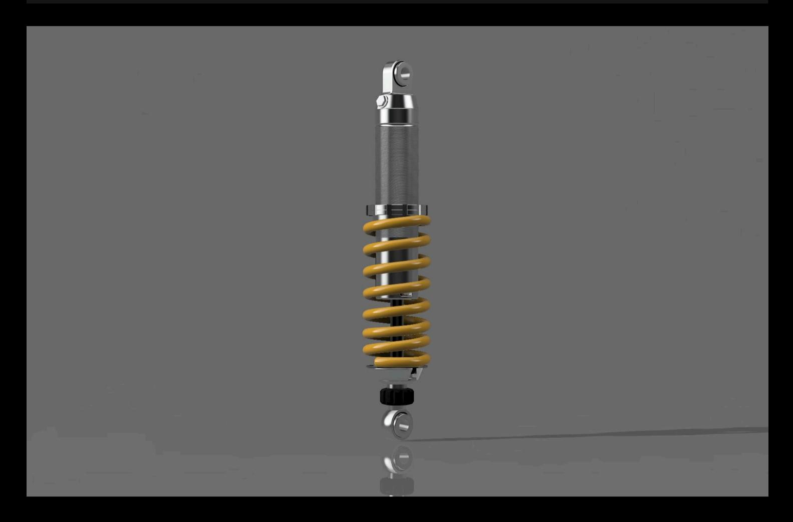
The custom high-pressure monotube gas shock absorber features an internal gas reservoir integrated into the main body. This design ensures compactness, stable gas pressure, and improved damping of road irregularities, resulting in efficient performance and durability in advanced suspension systems. The shock absorber is compatible with our front suspension systems: Bolt-On and Trapez Billet.
